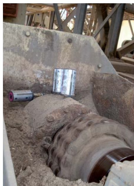
Lubrication of a chain drive with simalube
