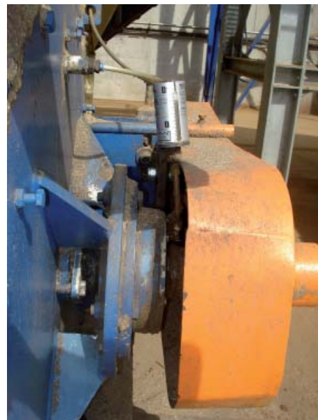
Lubrication of a bearing drive with simalube
