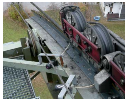
simalube ® with protective cap lubricating cable pulleys.
