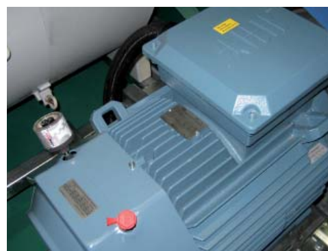
A 30ml simalube ® lubricator greases a compressor.
