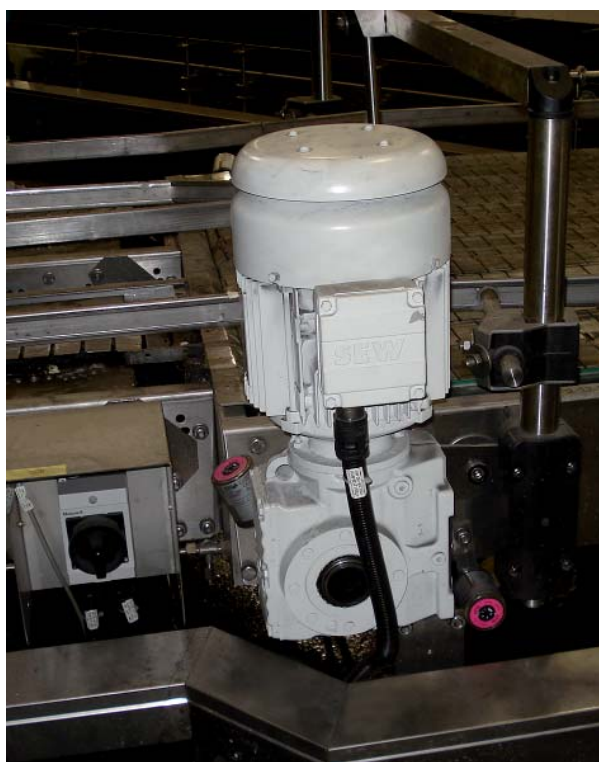
Driving motor with two greasing points.
