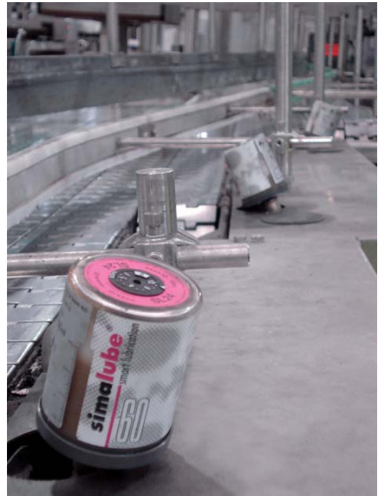
KRONES bottling line with simalube ® grease dispensers.
